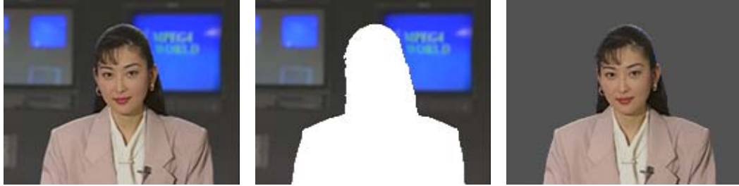
Figure 13: An example of video object (VO) concept in MPEG-4 video. A video frame (left) is segmented into two VO planes where VO1 (middle) is the background and VO2 (right) is the foreground.
