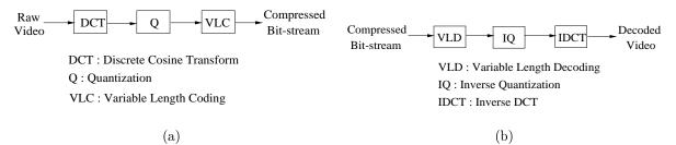
Fig. 6. (a) A non-scalable video encoder; (b) a non-scalable video decoder.
