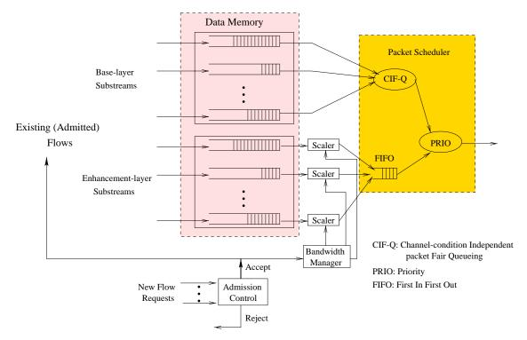
Fig. 13. An architecture for substream scheduling at a base station.
