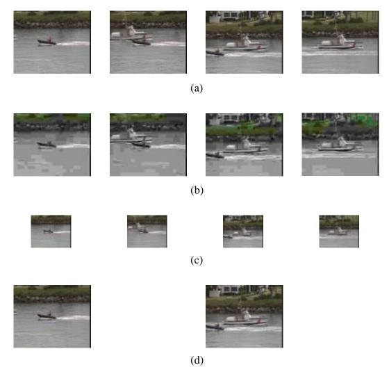
Fig. 5. Scalable video: (a) video frames reconstructed from the complete bit-stream; (b) video frames with degraded quality; (c) video frames with a smaller image size; (d) video frames with a lower frame rate.
