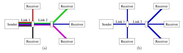
Fig. 1. (a) Unicast video distribution using multiple point-to-point connections. (b) Multicast video distribution using point-to-multipoint transmission.
