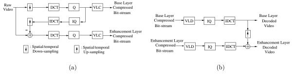
Fig. 8. (a) A spatially/temporally scalable encoder; (b) a spatially/temporally scalable decoder.
