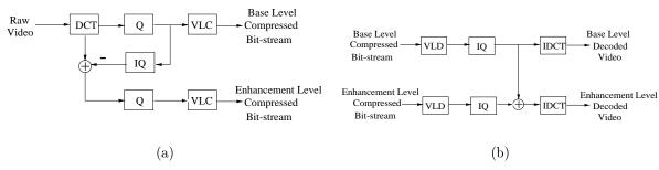
Fig. 7. (a) An SNR-scalable encoder; (b) an SNR-scalable decoder.
