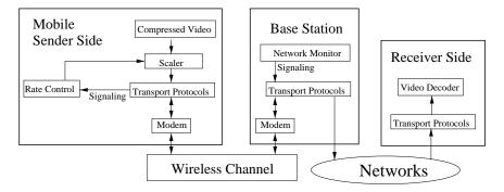
Fig. 10. An architecture for transporting scalable video from a mobile terminal to a wired terminal.
