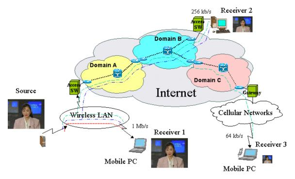
Fig. 3. IP multicast for layered video.
