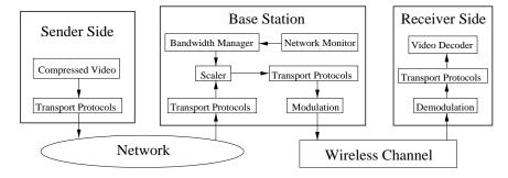
Fig. 11. An architecture for transporting scalable video from a wired terminal to a mobile terminal.
