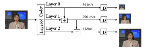
Fig. 2. Layered video encoding/decoding. D denotes the decoder.
